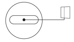
**3** Secure the webcam on your tripod by twisting it into the ¼ inch thread.
